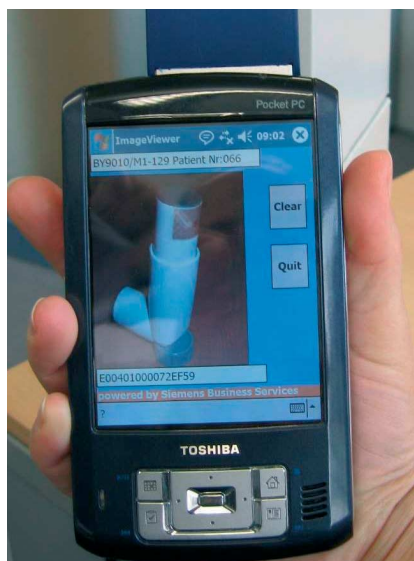
Fig. 4: Pocket PC with integrated RFID read/write compact flash card.
